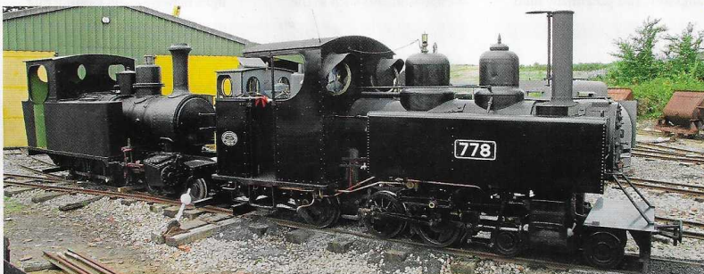
Surviving examples of the two types of 4-6-0T steam locomotives ordered by the War Department for use on the battlefield supply lines. To the right is Baldwin No. 778, restored to steam by the Greensand Railway Museum Trust. Left is Hunslet No. 303, owned by the War Office Locomotive Trust. The two were united for this August 31, 2009 picture at the Leighton Buzzard Railway's Stonehenge Works. The Hunslet, at that time a static exhibit, has subsequently been dismantled for restoration and should return to steam at the Pedale Valley Light Railway during 2015. CLIFF THOMAS
