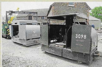
ABOVE: Two variants of 40hp Motor Rail Simplex locomotives resident at Leighton Buzzard. Left, WDLR No. 2182 (owned by the Greensand Railway Museum Trust) is an 'Armoured' type. The top elements of the 'armour' on No. 2182 are presently replicated in wood. It is planned to restore the loco both to operation and its full original appearance in metal over the next two years. It is seen coupled to WDLR No. 3098 (owned by the NRM) which is a 'Protected' type. CLIFF THOMAS
