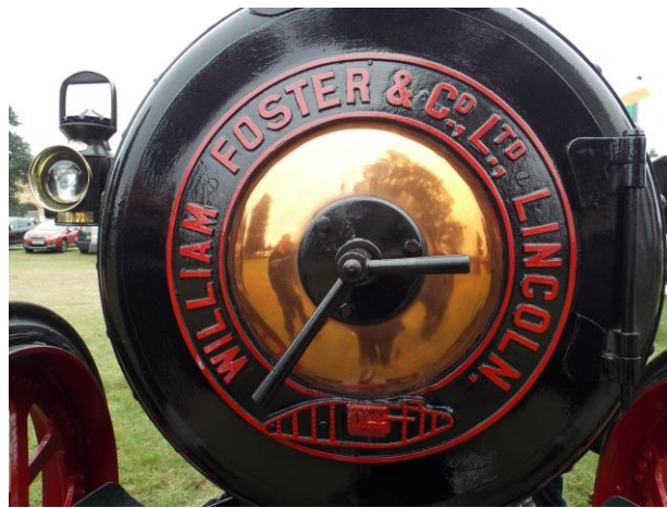
The William Foster and Co Ltd smokebox door ring showing the tank logo as fitted to one of their 1920's Fairground Showman's engine Photos: Tim Keenan
