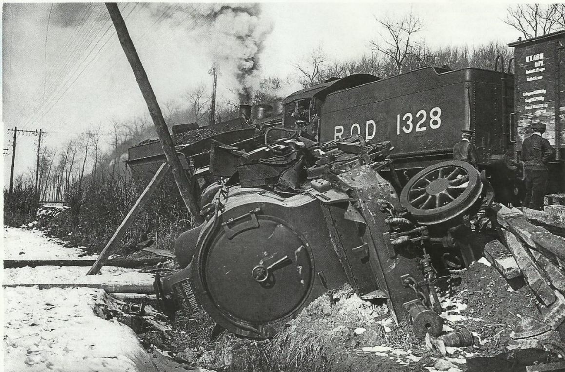
Mishaps on the Western Front were frequent, caused by direct artillery hits or by damaged track. Robinson 2-8-0 No. 1859 is passed by Baldwin 1328 at an unrecorded location. IWM
