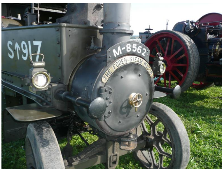
Front smokebox with special spring buffers on the Foden 7768 at the 2017 Great Dorset Steam Fair Image: Tim Keenan
