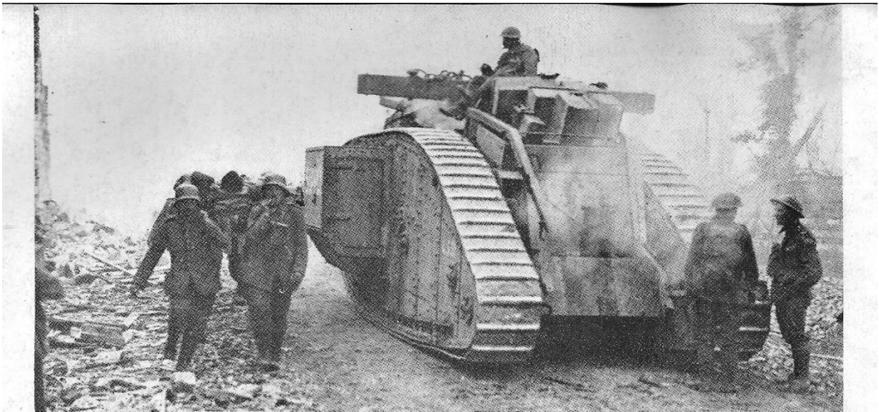
Supply Carrier Mk. IV clearly identifiable by widened sprockets and lack of armament.
