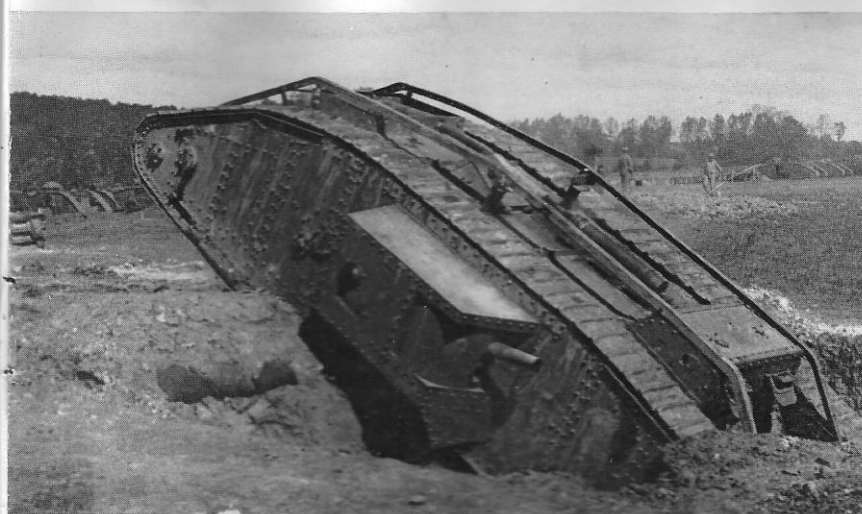
A Mk. IV dived in test pit at Tank Corps Central Stores, Erin, N. France, September 1917. Note single sponson turret, short 6 pdr. and machine gun ball mounting of this male tank.
