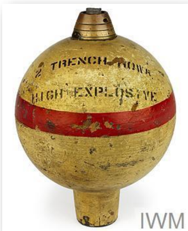
First World War period British trench mortar bomb. The 2-inch Vickers Medium Trench Mortar, also known as the 2-inch Trench Howitzer, came into use in the First World War in late 1915 but was phased out in late 1916. The term '2-inch' refers to the diameter of the mortar barrel, into which the bomb spigot (not shown here) was inserted, and the various types of bomb weighed between 39 - 42lb, with a range of up to 500 yards, depending on the size of the cordite charge used. For obvious reasons, this type of bomb was often nicknamed the 'Toffee Apple' or 'Plum Pudding' but sometimes also the 'Football'. © IWM MUN 3158
