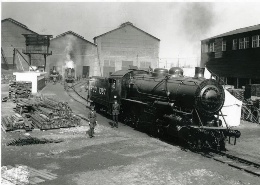
**The South Yard in ROD depot at Saint Etienne in France with American Baldwin 2-8-0 locomotive No.1397. Two Belgian 0-6-0 locomotives can be seen in the distance.**
