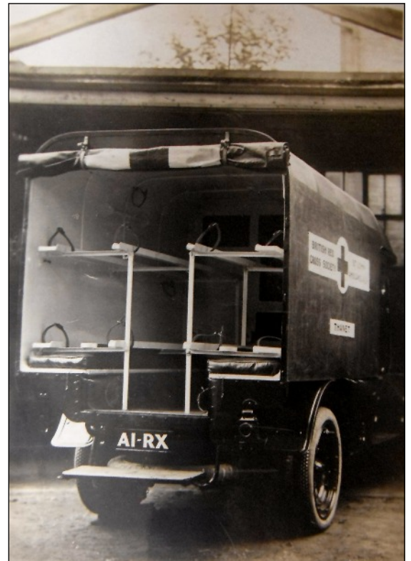
These two images show the interior of the “Thanet” Ambulance. The image on the left shows the ambulance’s four stretcher-supports folded and the step at the back of the ambulance in the ‘up’ position; and the image on the right shows the ambulance’s stretcher-supports ready for use and the step in the ‘down’ position
