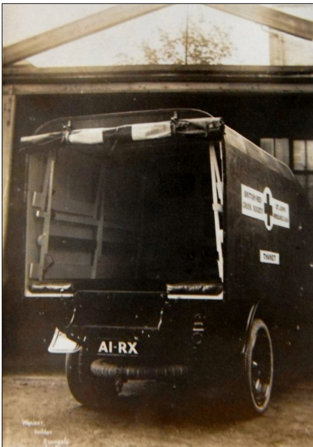
These two images show the interior of the “Thanet” Ambulance. The image on the left shows the ambulance’s four stretcher-supports folded and the step at the back of the ambulance in the ‘up’ position; and the image on the right shows the ambulance’s stretcher-supports ready for use and the step in the ‘down’ position
